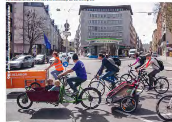
FIGURE 1 Free cargo bikes in Stuttgart, Germany. In the center, one of the most common models of cargo bikes – a two-wheeled cargo bike (in combination with an additional trailer); to the left, a three-wheeled cargo bike with an orange box.
